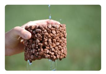
Proper maintenance of pervious concrete starts with good design to prevent clogging. We recommend at least an annual infiltration test to determine what type of maintenance is needed or if it is needed. As with many things, "an ounce of prevention is worth a pound of cure," so keeping the pavement surface free of dirt and
