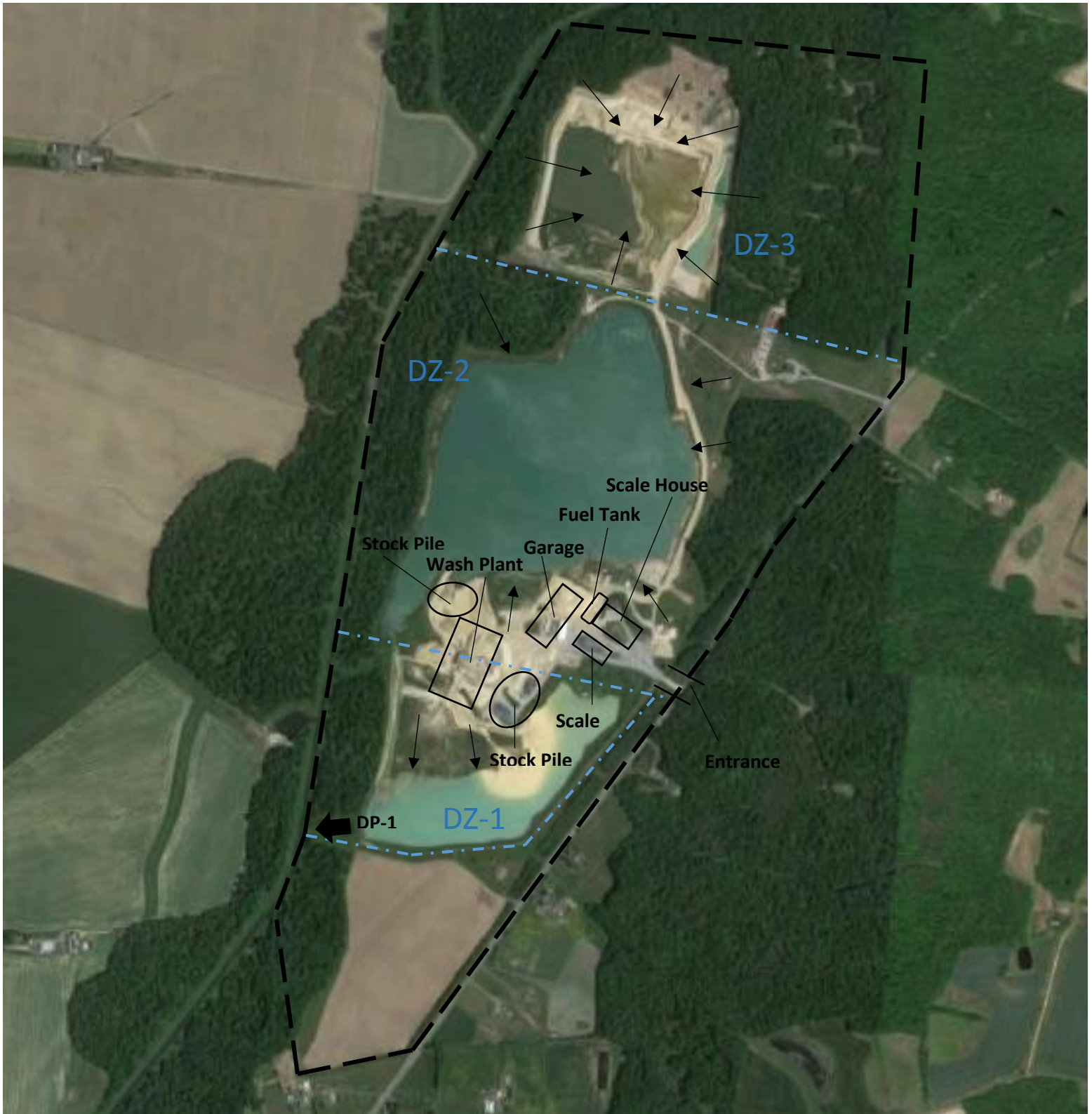
FIGURE 2 FACILITY SKTECH OF EXISTING CONDITIONS
